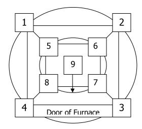
For vertical furnaces, (9) T/C's shall be placed at 120° positions at the bottom, center, and top levels of the hot zone located at the outside extremes of the work zone. Also, (1) additional T/C shall be located at the center position of the work zone.
