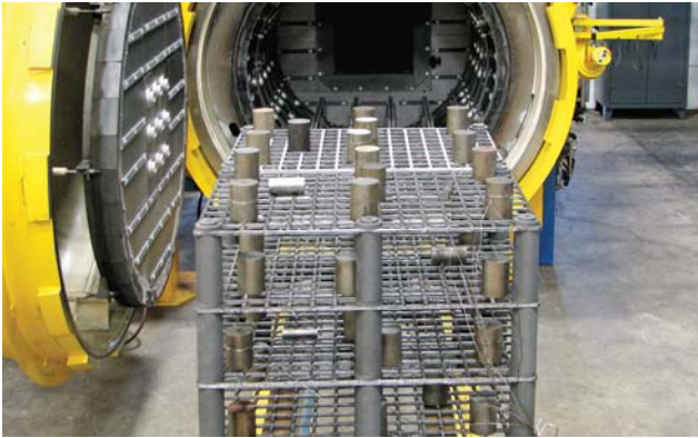
Fig. 5. C/C test-fixture assembly with test pieces
