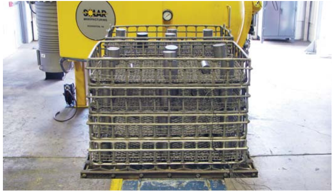
Fig. 6. Alloy test-fixture assembly with test pieces
