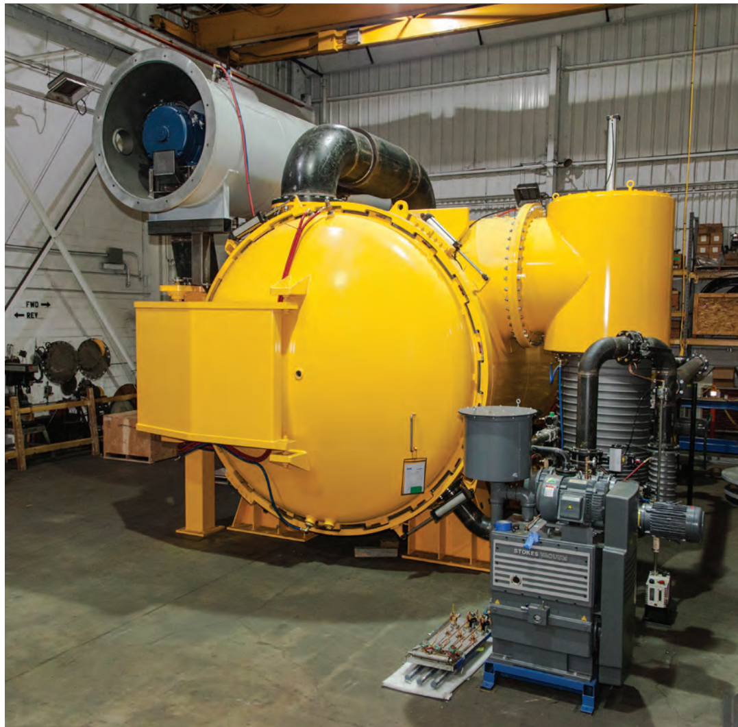
■ Solar Atmospheres of California's new furnace under construction in the Solar Manufacturing shop
