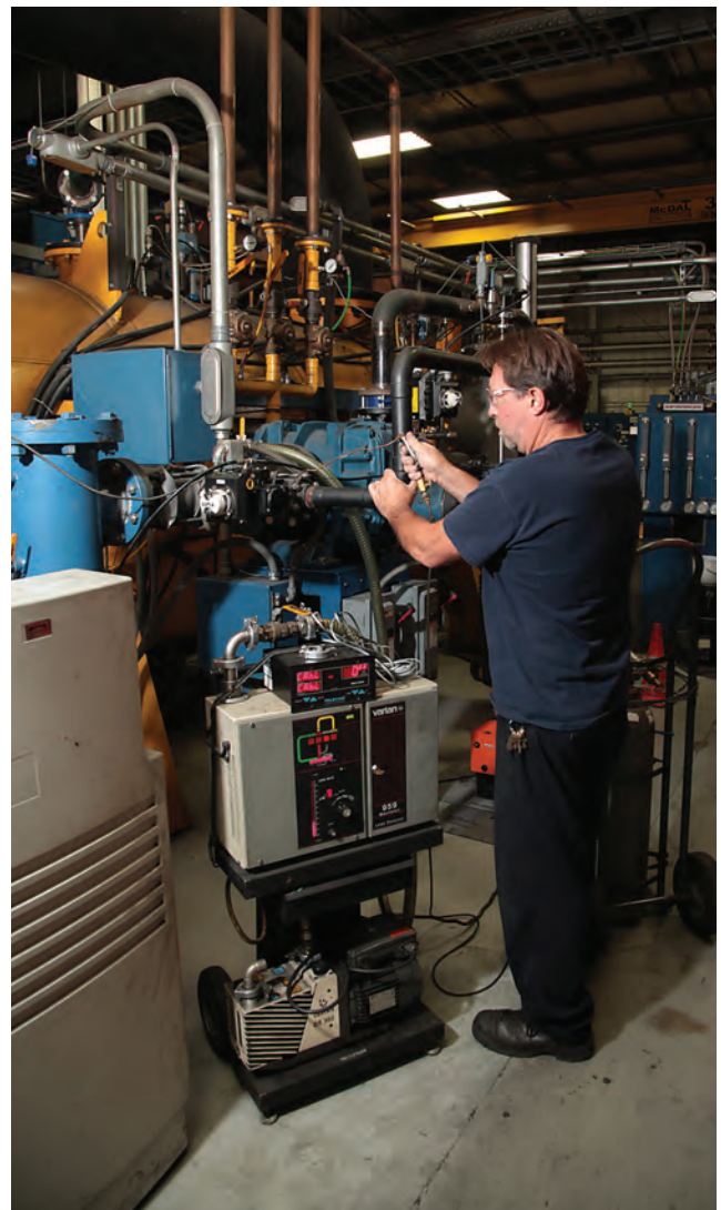
■ A technician using a Varian helium mass spectrometer to test for leaks at a pump valve.
