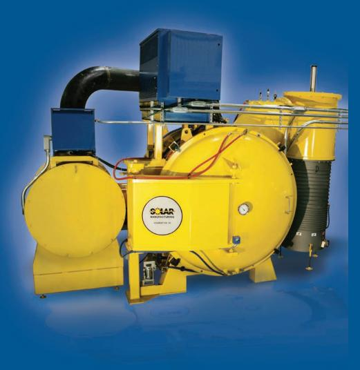
The HFL-EQ model is a horizontal front loading, external quench, vacuum heat treating and brazing furnace generally designed for high production commercial and captive heat treating shops. It is a high temperature, high vacuum, batch-type furnace with electric resistance heating elements. All aspects of form, fit and function are designed for easy maintenance and minimal downtime.
