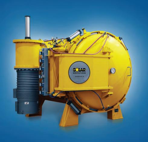
The HFL-IQ model is a horizontal front loading, internal quench, vacuum heat treating and brazing furnace generally designed for high production commercial and captive heat treating shops. It is a high temperature, high vacuum, batch-type furnace with electric resistance heating elements. All aspects of form, fit and function are designed for easy maintenance and minimal downtime.
