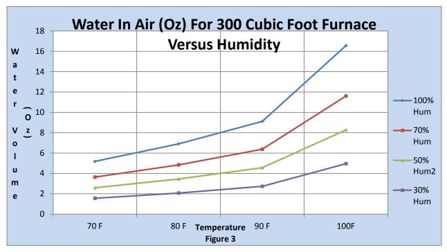
expected for various humidity levels and operating temperature conditions. This plot is shown in figure 3. Typically, as is shown, when operating at a relative humidity of 70 % and an outside temperature of 90  $^{\circ}$ F, we would have to pump out approximately 6.25 ounces of water.
