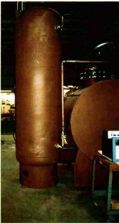
Fig. 4 Inert gas in reservoir tank for vacuum heat treating furnace can be measured for moisture by electrolytic hygrometer.
