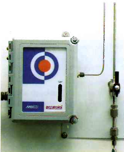
Fig. 2 Measurement for moisture of incoming gas supply is determined by this hygrometer.
