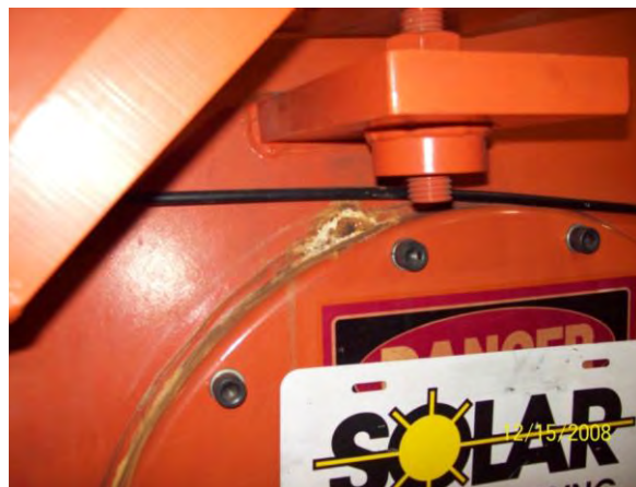
Figure 11 - Seam Weld Problem
