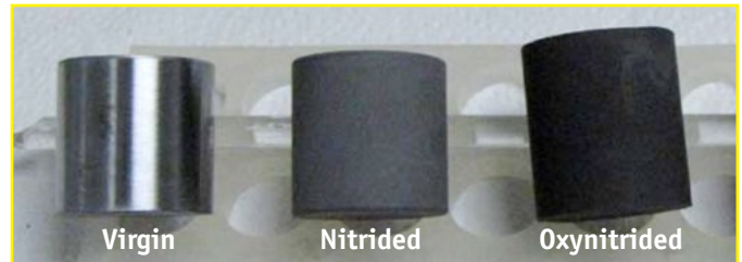
Before salt spray testing
