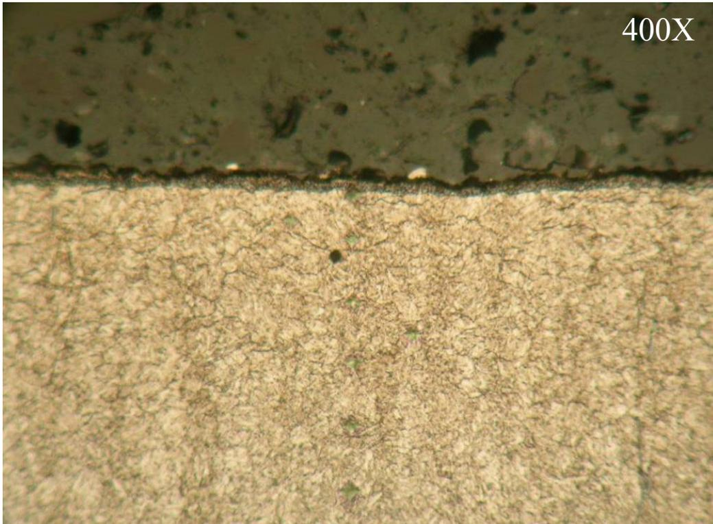
Figure 6a: Microstructure of 80 minute nitrated material after 2 hr diffuse
