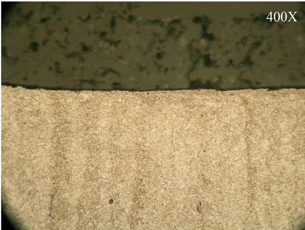
Figure 7a: Nitriding for 20 minutes after surface washed with alcohol only
