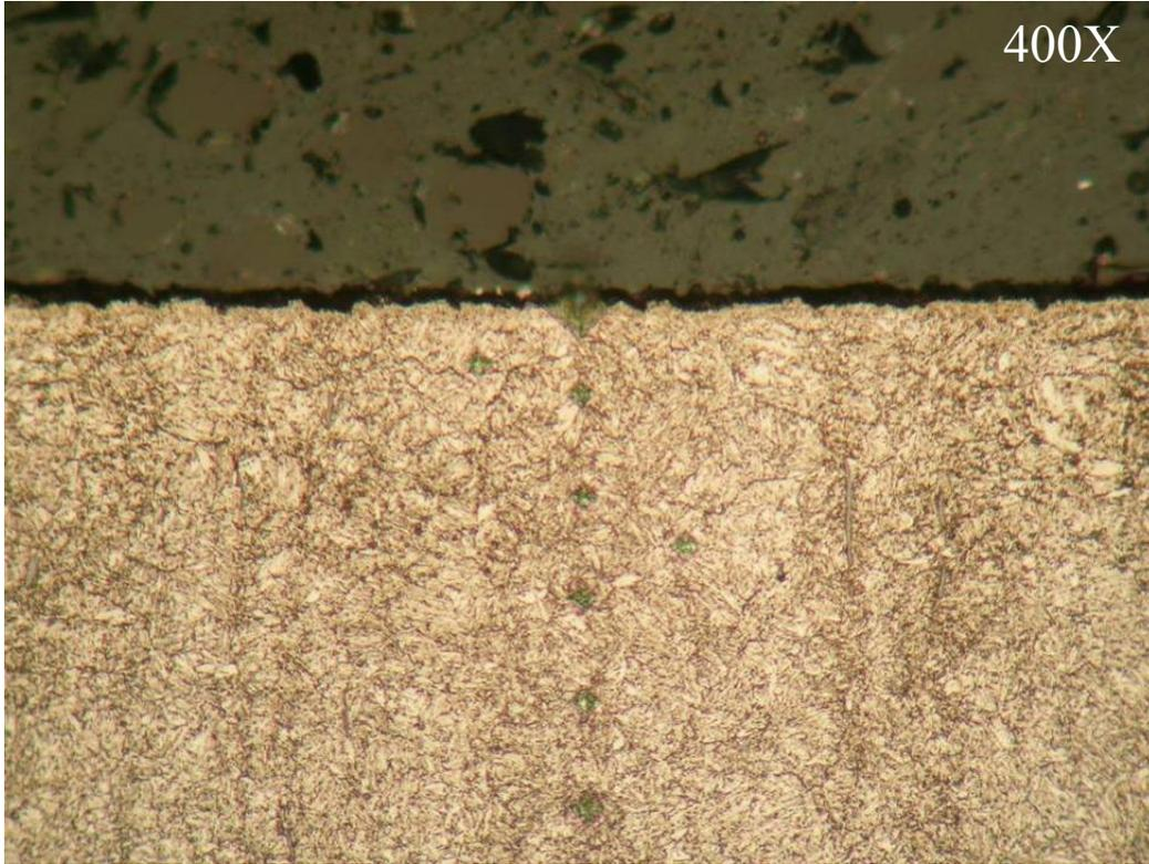
Figure 6b: Microstructure of 80 minute nitrated material after 4 hr diffuse
