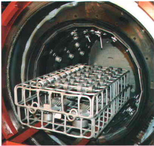
Fig. 5. Production furnace refitted with carburizing controls for vacuum carburization
