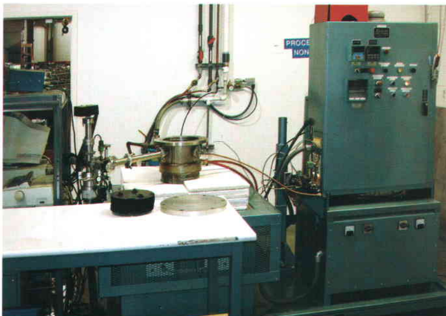
Carburizing development starts out small in lab-scale retort furnace and finishes big (in production scale furnace; see Fig. 6)
