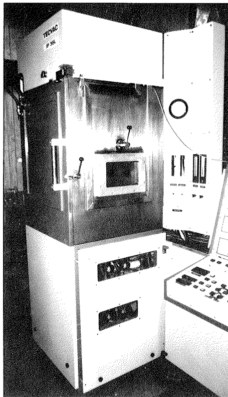
Fig. 1 Coating chamber of ion plating unit.
