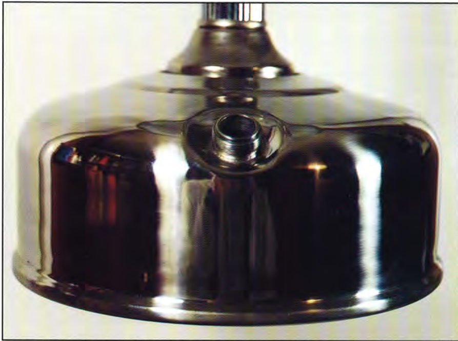
Fig. 2 Nickel brazed lamp oil tank vacuum furnace brazed along the bottom seam and at the spout.
