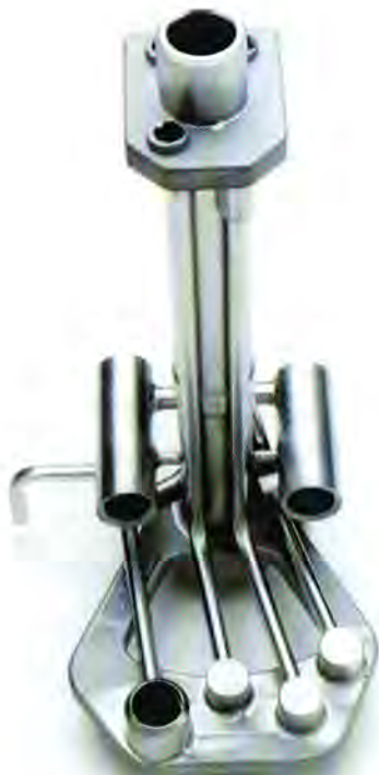
Fig. 4 Nickel brazed assembly showing the variation in components—tubing, cast and machined.
