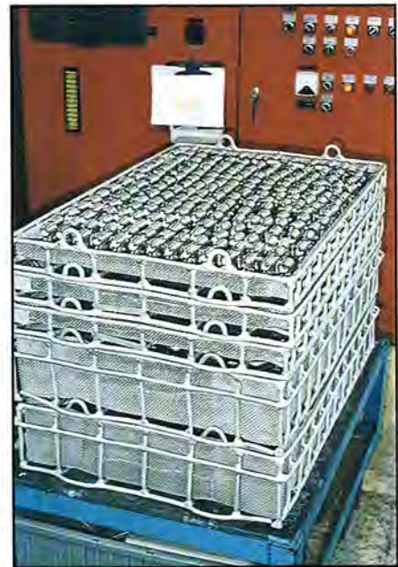
Fig. 5 Production run of assemblies in layered baskets ready for brazing and heat treatment in vacuum furnace. Control panels are shown in background.
