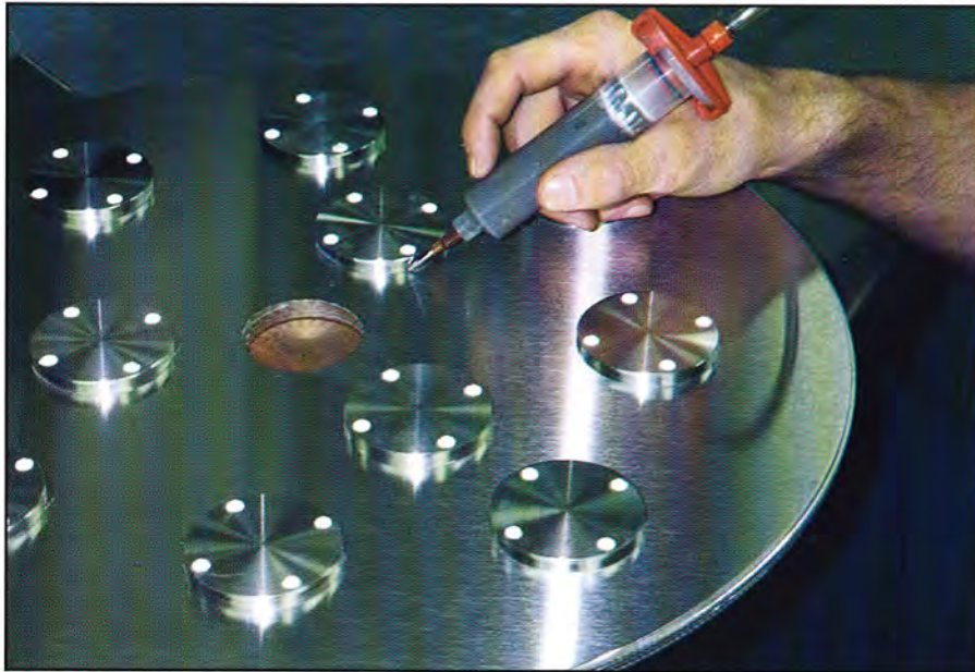
Fig. 3 Pneumatic, needle point, application of braze alloy to components.
