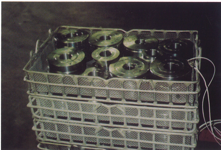
A basket, constructed of alloy rod and lined with wire mesh, holds small pieces ready for the furnace.
